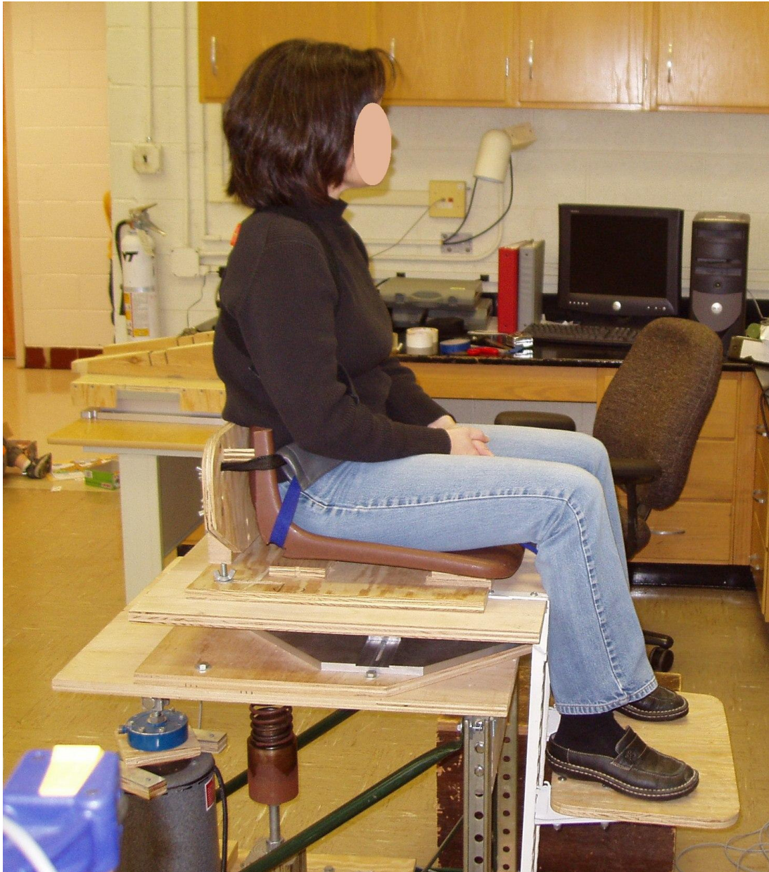
Figure 3.1: Participant balances on the wobble chair moving the lumbar region of her torso to maintain stability.
