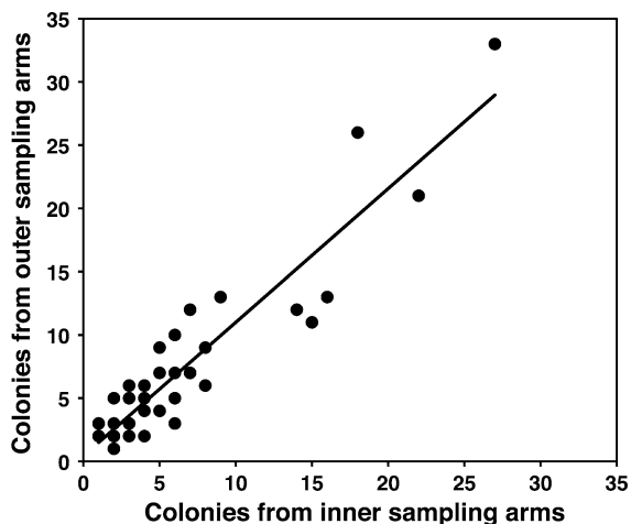
Fig. 3 Scatter plot and simple linear regression of consecutive sampling of Fusarium with inner (4 plates) and outer (4 plates) arms of a UAV. A significant correlation ( r = 0.93 , P < 0.001 , n = 98 ) was observed between colony counts of Fusarium from the inner and outer arms. Flights were conducted 100 m above ground level during 2010 and 2011. Flights F207 and F208 were outliers and were removed from the analysis
